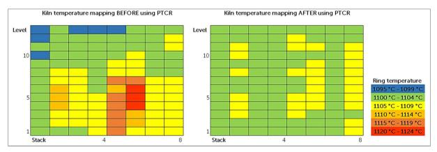
The most frequent use of PTCR is by optimising and managing the firing/sintering processes to achieve the optimal product quality and to assess the thermal performance and characteristics of a kiln/furnace. The way of working is to make a number of runs with different settings of the parameters temperature and time. These runs are characterised by the ring temperature (RT) values as determined from the rings. Product quality analysis determines the optimal run and accompanying RT values.
